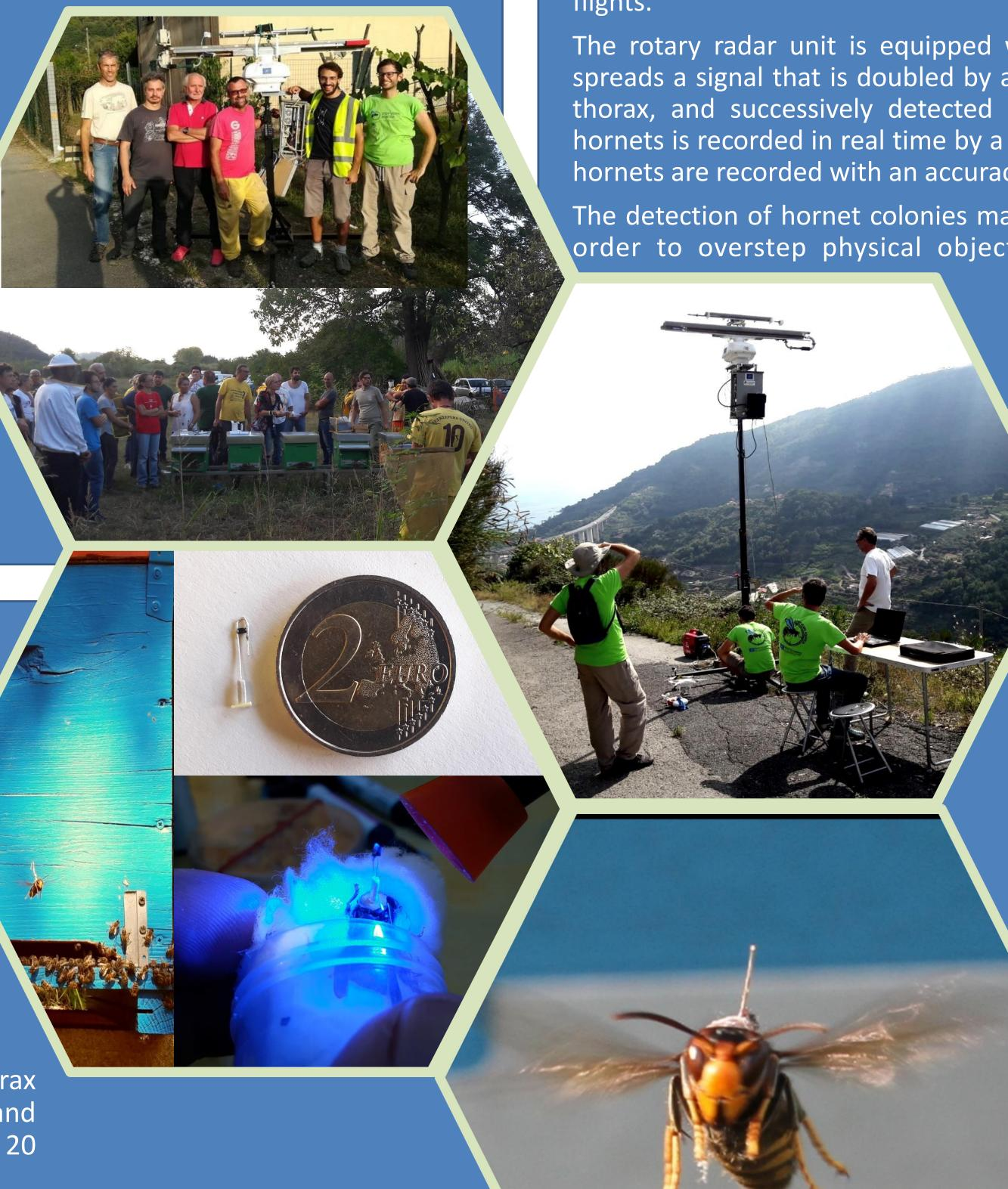
The harmonic radar allows to track the flights of foraging hornets equipped with a small passive transponder (tag), in order to detect the position of the colonies they came from. The small dimension and lightweight transponder provides various advantages in terms of maintenance of flying capabilities, allowing tagged hornets to continue successfully their foraging activities, enabling operators to track both nest-returning and outgoing flights.
