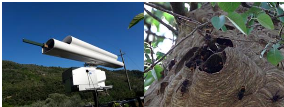
Figure 8 - Second prototype of entomological harmonic radar (left) developed by LIFE STOPVESPA for locating V. velutina nests (right). Two tagged hornets are present near the entrance of the nest.
